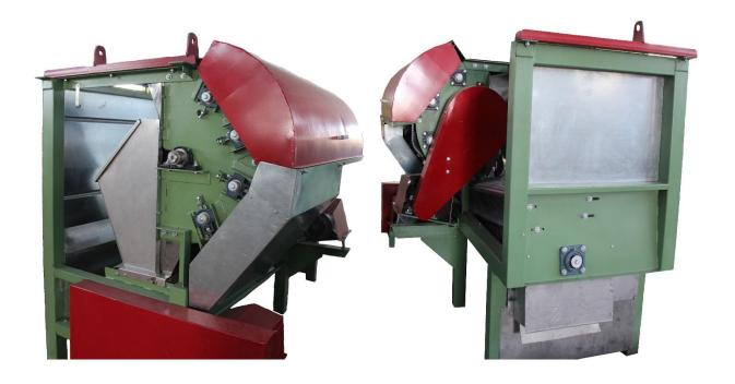
This machine is used for hulling the fresh product. The principle is that by rubbing the product between two rubber drums, with different speeds, the product's hull will be removed.
