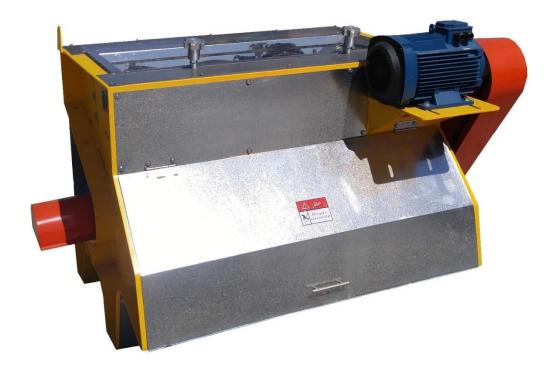
This machine is used for hulling the fresh product. The principle is that by hitting the product with some bolts, fasten to a drum, the product's hull will be removed. This machine is rougher than a rubber hulling machine so it can be used for hulling the stick tight pistachios. A percentage of kernel in the output is normal.
