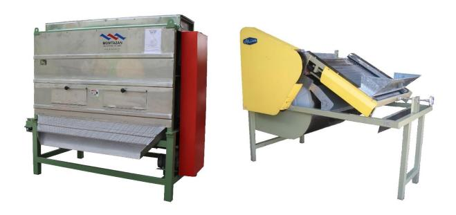
This machine separates hulled pistachios from unhulled pistachios. Pistachios are separated in this machine by the difference in their friction.
