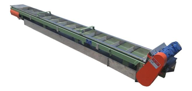
This machine is used for transferring pistachio in processing line. The small bagged model uses for elevated fresh pistachio from orchard and another one is used for elevated hulled pistachio between two machines.
