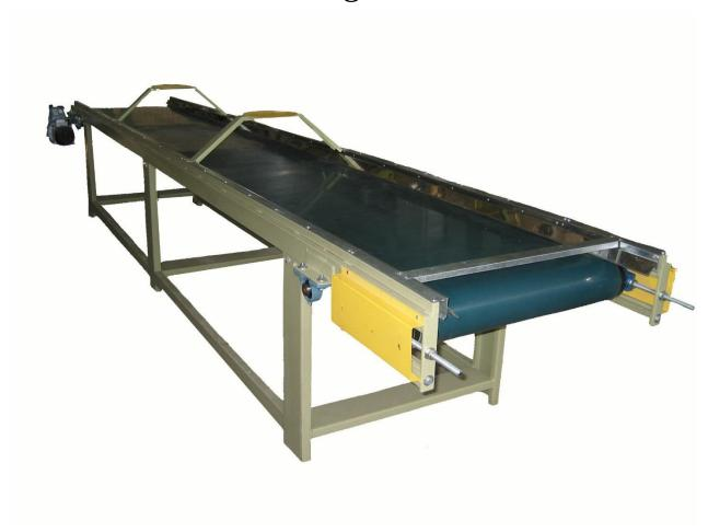
This machine is used in end of pistachio processing line. And some workers sit down side of a wide belt for separating unsuitable pistachio from good pistachio.
