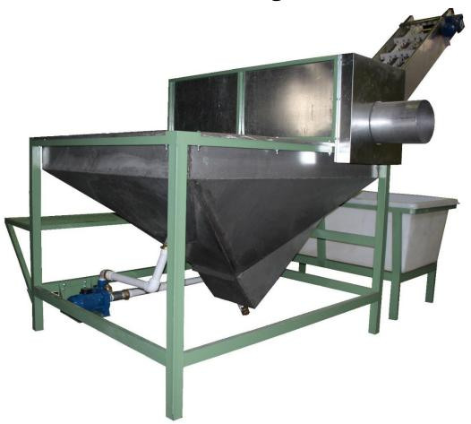
After the product exits washing system, it enters this machine and the output goes to the pre-drier. The main function of this machine is to remove the light products from the heavy ones with the help of water. The light product will float on top of water and will exit from the side of the machine with the help of screw conveyor, but the heavy and good product will be taken out from the bottom of the tank with the help of a polyethylene chain conveyor.
