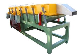
The main function of this machine is to remove the light and blank pistachio from the heavy ones with the help of Air. The blank pistachio will be floated and exited from the side of the machine. the heavy and good product will be out from the end machine. Also, this machine separates tiny pistachio, dust and trash from good pistachio.
