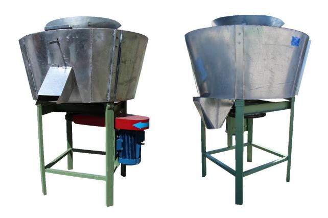
After the product exits the hulling system, there is some unripen pistachio and they must be peeled so they will be entering the hulling unripen machine to be hulled them. The pistachio is peeled with screw and water.
