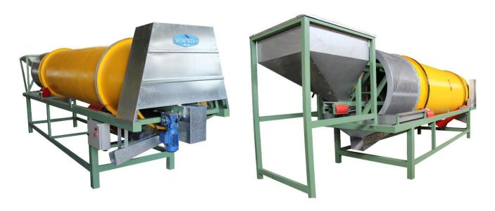
This machine is used for separating open mouth pistachios from close mouths. This machine includes a big rotating cylinder that some special needle belts installed in it. While feeding the drum, the open mouth pistachios are carried on by the needles and then fall in a belt conveyor by a brush but the closed pistachio because they cannot be caught by needles, they will go out of the end of machine.
