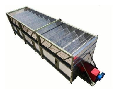
This machine is used to dry the fresh product completely. The system used in this drier is a complete-discharging system. The hot air needed for drying and it is produced by a heat exchanger which works with gas or diesel.
