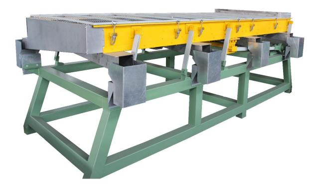
This machine used for separating different size pistachio from each other. This machine separated pistachios in different size with using different perforated plate and the pistachios move to forward by vibration.
