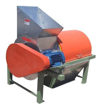
This machine is used for removing bunches from the fresh product. The product which comes from the orchard is usually in bunches, so this machine is necessary for removing bunches and sticks from the main product. The output of this machine will enter the hulling machine. In the next stage for a 6 ton model the hull and small bunches are removed by a helical drum. This helical drum also moves the product forward while removing the trash from it.
