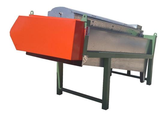
After the product exits the hulling system, it will enter the washing system to be washed. While being washed small bits of hull will be also removed from the product. This machine is design so it can reduce the water consumption. For this purpose, a Helical drum is used, while the product is washed with some sprayers it is moved forward and also stirred so the washing efficiency increases.
